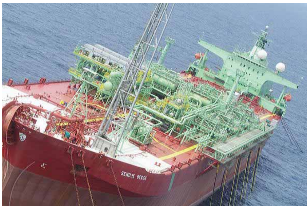
An FPSO vessel with processing facilities on deck and risers coming in on its left.
